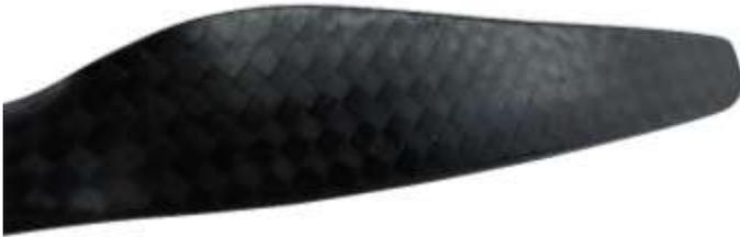
Carbon fiber reinforced plastic (CFRP): CFRP's are used in various applications with high demands regarding strength and light weight. They consist of two main components: Carbon fibers and the surrounding plastic holding together the fibers.
