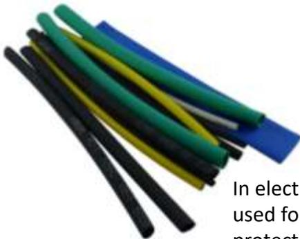
In electrical engineering, heat-shrink tubing is used for electrical insulation and environmental protection for conductors, joints, and terminals. The plastic tubes shrink radially when heated, enclosing the protected components.
