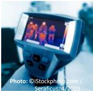
In a thermal imaging camera, special sensors pick up the invisible heat radiation of an object and convert the information into electrical signals, based on the measured heat intensity. In this way, temperature differences in and around an object can be shown by the thermal image.
