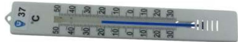
Liquid expansion thermometers were the first instruments that could deliver accurate temperature measurements. A thermometer measures temperature changes based on the thermal expansion of a liquid (e. g., mercury).
