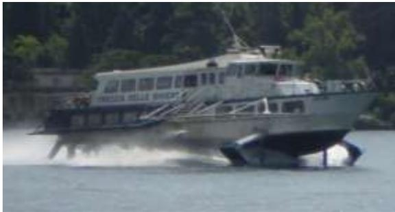
Unlike conventional boats, the hull of a hydrofoil is lifted out of the water when traveling at speed in order to reduce drag.
