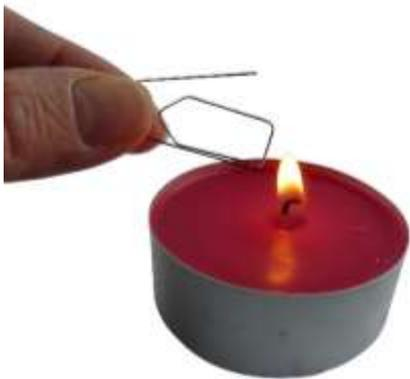
Heating a shape memory metal initiates a phase transition, which causes the metal to change to its original shape before it was deformed.
