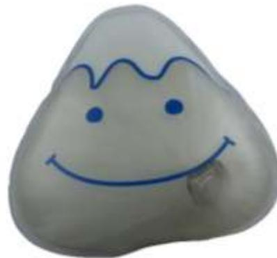
Instead of hot water bottles, which need to be filled before use, gel-based heat packs use the latent heat of fusion. A metal plate triggers the phase transition process (crystallization) when pressed, and this process generates warmth. These types of heat pack can be recharged by immersion in very hot water until the contents are fluid again, and then being allowed to cool.
